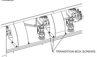
FIG. 57 Loosening Fan Transition Box Screws
